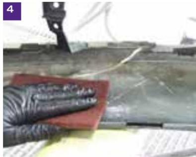
Abrade the area with a BDPBWPBUF Bodyline red or grey weave pad removing all dirt and overspray.
