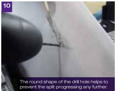
Drill a hole at the end of the crack as seen in the picture using a 3mm drill bit.
