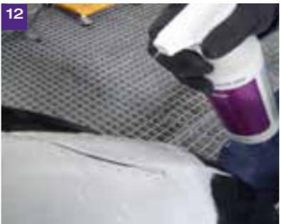
Apply Bodyline Plastic Cleaner BPC500 to the outside and inside of the panel and clean with a Bodyline pre-cleaning cloth BDPBPCC.
