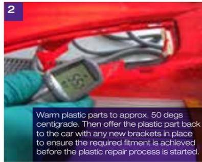
If required, heat the plastic part with an Infra Red unit or a heat gun to assist the part to return to its original profile.
