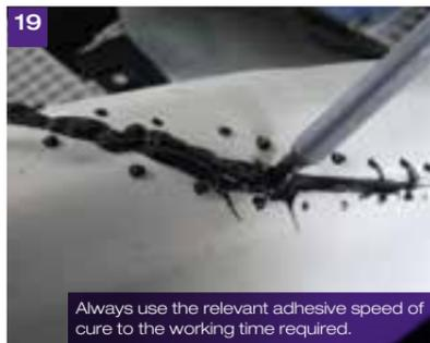
To fill the gap to provide the required profile, apply adhesive keeping the end of the nozzle buried in the adhesive.
