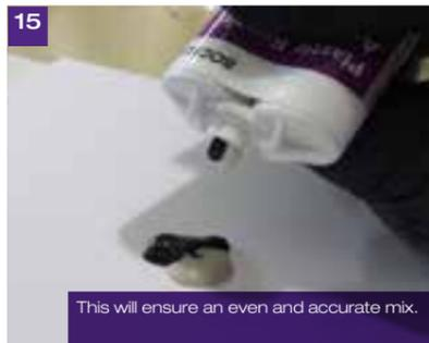
Purge the tube before attaching the mixing nozzle as per the picture.
