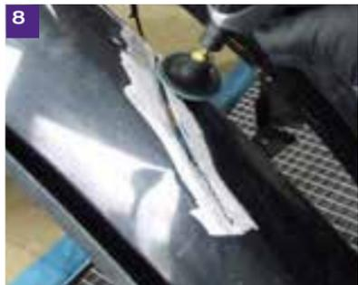
Create a shallow V next to the split both inside and outside of the panel with a Bodyline Griplock Disc to provide adhesive strength to the split panel.
