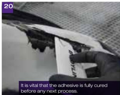
Smooth and place the adhesive to the required profile using a Bodyline plastic spreader (BDPBFBFS).
